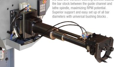
The Marubeni Citizen-Cincom C-332 is designed for automatically feeding round, square and hexagonal bar stock in lengths up to 12', in a diameter range of 3-32 mm, into CNC lathes.
