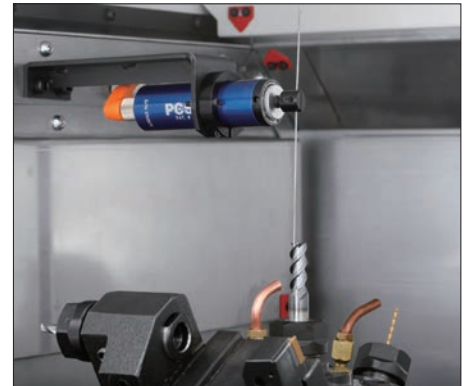
Drill breakage detector (option) Drill breakage is detected by the swing cylinder. The machine stops when breakage is detected, and a second accident can be prevented.
